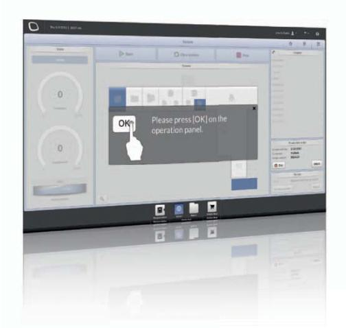
Thanks to the application **Recipe** the user – for the first time – is no longer required to program any machine functions, instead he only has to describe the characteristics of the material to be processed. This means that detailed knowledge of the system is no longer required. A recipe consists of pre-defined material modules (e.g. documents, enclosures, envelopes). Recipes are created independently from the inserting system and may be processed on different inserters.
